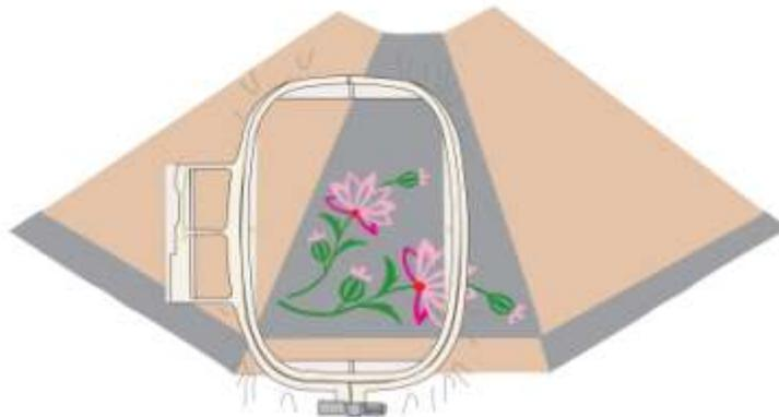
3. Click on the Camera icon on the machine. The machine will scan the fabric in the hoop. When the scan is complete the fabric and the embroidered design will appear on the screen.
