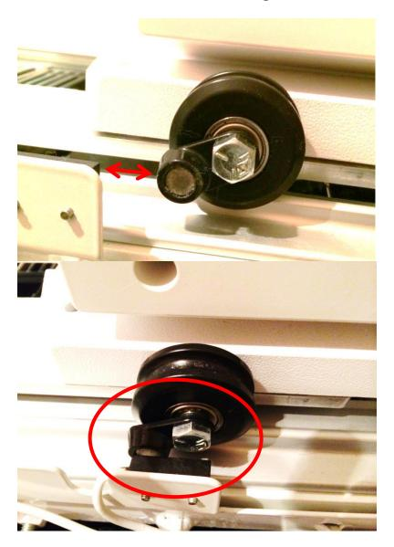
5. Move the machine forward so the magnet passes the sensor and the idle rail should move forward. Then move the machine back and the idle rail will move back. It may take several times for the two sides to calibrate and be in sync with each other.
