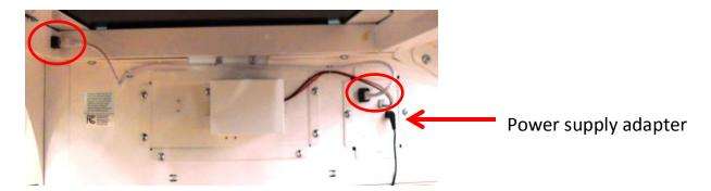
Connect the cables on the left side of the frame. These also are taped to the inside of the frame. There is no power supply on this side.
