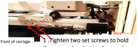
1 .Tighten two set screws to hold the sensor bracket in place and peel the two sided tape at the back end of the bracket and press it to the carriage. 2. Attach the master board box using the two sided tape to the sensor bracket. Plug the sensors into the correct port as marked on the box. Plug in the power adapter to the box.
