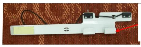
The bracket has two tabs that fit around the bottom edge of the carriage side rail.
