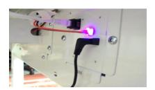
3. Plug in the power supplies. The light on the right will be red. Turn on the speed switch and the light should be blue and red. The blue light means the boards are communicating. The light on the sensor bracket board will be red.
