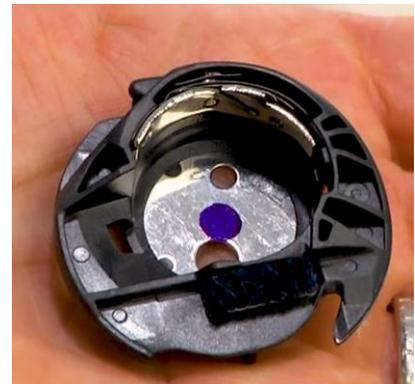
When using pre-wound bobbins, if the height is lesser than the Class 15 bobbins that came with your machine, use the center pin to make the bobbin the same height as the Class 15 bobbins.
