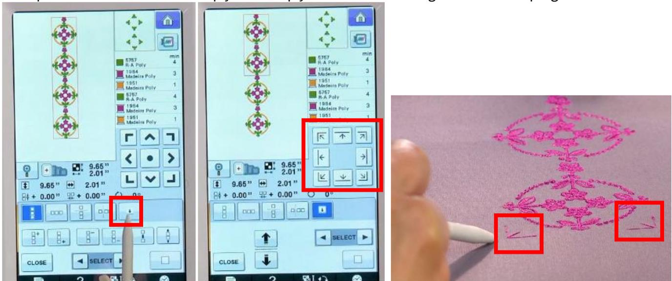
Use the alignment keys to line up the top corners of your design (make sure the needle is lined up with the justification – check the top left of the design and the top right) to make sure they align with the registration stitches on the fabric from the previously stitched design.
