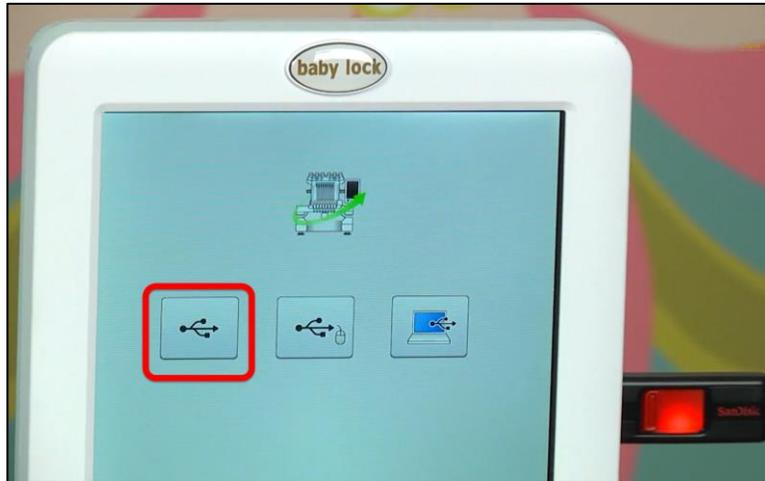
7. A new screen is displayed which tells you to “Press Load after connecting the USB media containing the upgrade file.”
