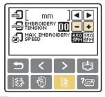
Press - to weaken the thread tension.
