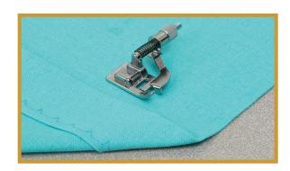
3. Place fabric so that the straight stitches are on the extended hem edge and the zig zag stitches just catch one thread of the folded edge. Turn the screw so that the guide barely touches the folded edge of fabric.
