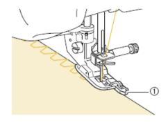
**Note:** After the stitch width is adjusted, turn the handwheel toward you by hand and check that the needle does not touch the presser foot. If the needle hits the presser foot, the needle may brake and cause injury.
