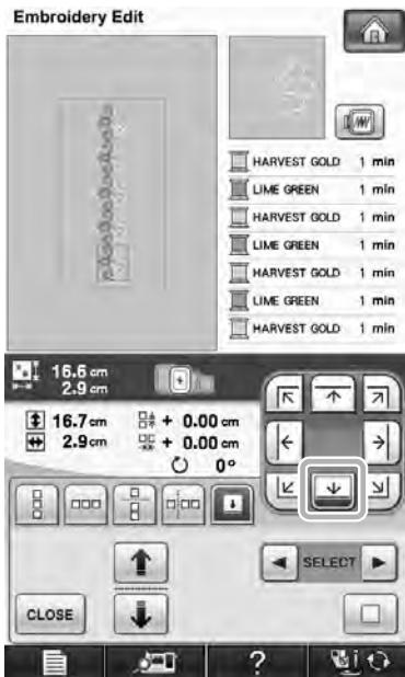
→ Touch **↑** and **↓**, or **←** and **→** to highlight the design for inserting thread marks.
