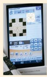
Precise placement is easier than ever. Using the NeedleCam, a scan of the fabric in the embroidery frame can be displayed on the LCD so you can preview where your embroidery designs will be placed, even in tricky places like collars and hems, or for centering designs within quilt blocks.
