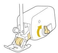
When the feed position lever is down, the black roller belt on the dual feed is engaged.
