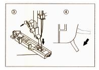
4. Position fabric under presser foot so that the center line mark is in the center of the needle opening in the buttonhole foot. With the main part of the foot
