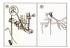
9. With the buttonhole cutter cut the center of the buttonhole being careful not to cut the stitches on either side. Use a pin as a stopper.
