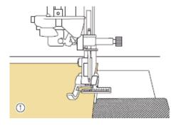
7. When the Built-In Camera detects the edge of the fabric, the fabric edge indicator line (2) appears correctly following the edge of the fabric.
