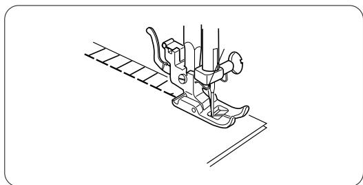
Overedge stitch will be done most successfully when the right side stitches of zigzag fall slightly off the edge of the fabrics.
