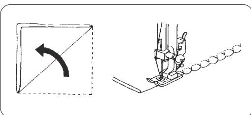
Place the bias folded edge of fabric along the inside right edge of the needle slot of foot.
