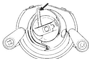
Raise the needle by turning the handwheel toward you.
