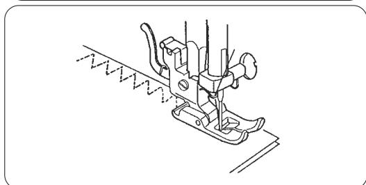
Place the fabric under the presser foot so that the edge is just inside the right edge of the presser foot. Guide the work so the right hand stitches fall off the edge of the fabric.
