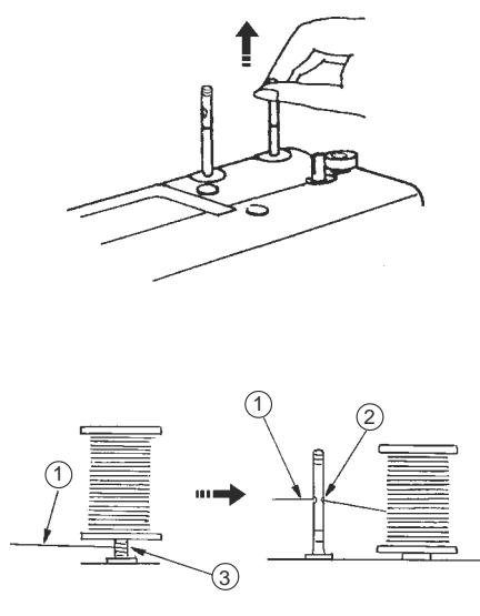
The spool pins are used for holding the spool of thread in order to feed thread to the machine.
