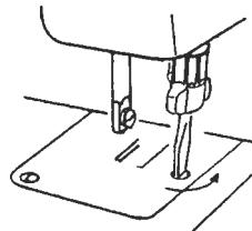
Remove the needle and the presser foot.
