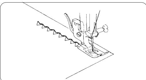
If forward and reverse feeding becomes unbalanced due to the type of fabric, adjust the balance by turning the stitch length dial as follows:
