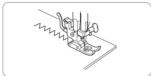
Simple zigzag stitching is widely used for overcasting, sewing on buttons, etc.
