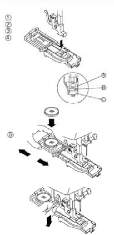
14. When buttonhole sewing is finished, push the buttonhole lever upward as far as it will go.
