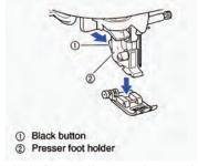
Use the included screwdriver to loosen the presser foot holder screw, and then remove the presser foot holder.
