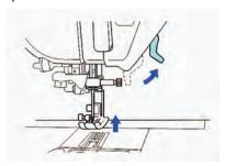
4. Press the black button on the presser foot holder to remove the presser foot.
