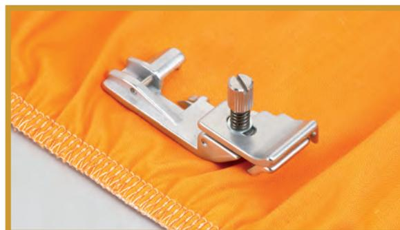
Attaching Elastic using the Elastic Foot:
