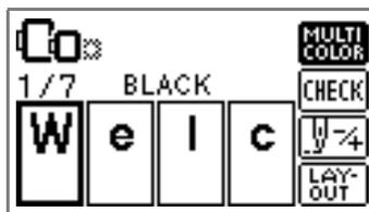
**U-74** The needle progresses one color or one stitch (if pressed continuously, 9 stitches to 20 stitches) at a time and changes the position for starting the embroidery. This is used when a specific color is not sewn or when restarting the sewing machine after power has been turned off in the middle of the operation.
