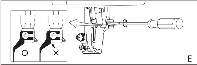
5. Slide the new latch wire onto latch wire screw until the opening is completely against the screw. Securely tighten the latch wire screw. (Fig. E)
