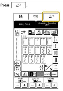
→ The screen changes, and all keys and operation buttons are locked.
