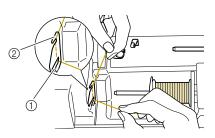
Lower notch in the thread guide plate
