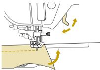
The pivot setting is useful when changing the sewing direction. When the machine is stopped at the corner of the fabric, the machine stops with the needle in the fabric and the presser foot is automatically raised so the fabric can easily be rotated (see "Pivoting" on page 45).
