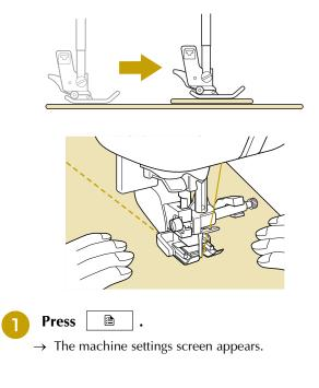
Press to display P. 2, and then set the "AUTOMATIC FABRIC SENSOR SYSTEM" (Automatic Presser Foot Pressure) to "ON".
