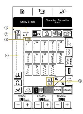
(1) Shows whether the machine is set for a single needle or twin needle, and the needle position when the machine is stopped. The desired needle position can be set (see page 20).
