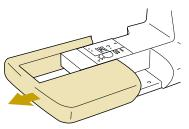
→ With the flat bed attachment removed, free-arm sewing is possible.
