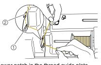
1 Lower notch in the thread guide plate Upper notch in the thread guide plate While holding the thread from the spool in your right hand, hold the end of the thread with your left hand, and then guide the thread through the groove, following the arrows in the illustration.
