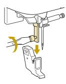
Position the free motion echo quilting foot 5 "E" on the left side of the presser bar with the holes in the quilting foot and presser bar aligned.
