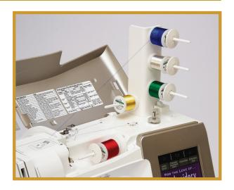
3. When threading the machine from the tower, make sure the thread is coming off the bottom of the spool. Use one of the provided spool caps, or one provided with your machine to secure the thread spool in place.
