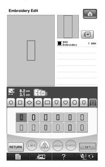
When the pattern connection setting screen (screen for connecting the selected pattern to the previous one) appears, select the reference edge and reference point for connecting the first pattern, and then press ok. Since, in this example, we will connect the center point of the top edge for the second pattern with the center point of the bottom edge for the first pattern, select the center point of the top edge, and then press ok.
