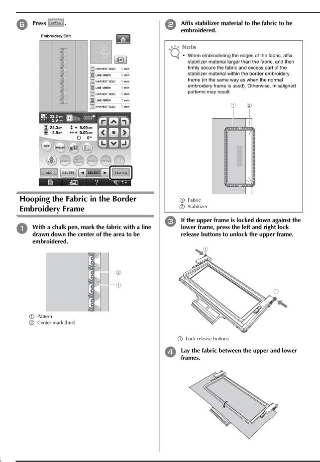
Place the embroidery sheet in the upper frame, align the center mark (line) on the fabric with the guide line on the embroidery sheet, and then press down on the left and right locking levers until they click into place.
