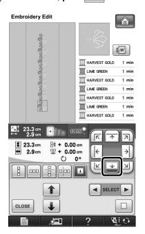
→ Touch 1 and 1, or 1 and ► to highlight the design for inserting thread marks.
