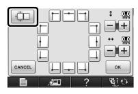
Select the new reference edge and reference point for connecting the pattern, and then press or.
