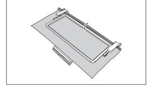
6 Remove the embroidery sheet, and then gently pull the four sides of the fabric to remove any excess slack. Be careful so that fabric is not stretched out of shape. Finally, check that the fabric is firmly within the hoop.
