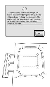
If the fabric cannot be rehooped so that the next pattern and the centers for the large circles of the two stickers are within the embroidering area, hoop the fabric with the centers for the large circles of the two stickers within the embroidering area and the next pattern as close as possible to being within the embroidering area, and then attach the frame to the machine.
