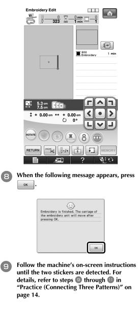
After the two stickers have been detected, the following message appears. With the stickers remaining affixed, remove the frame, and then press
