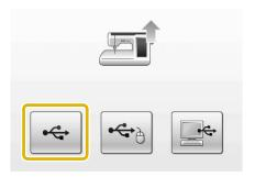
Insert the USB media into the primary (top) USB port on the machine. The media device should only contain the upgrade file.
