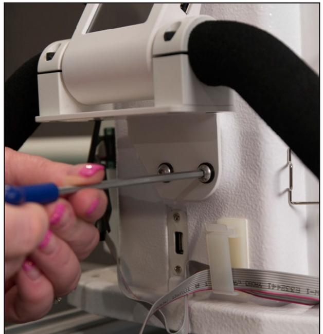
4. After the two bolts are in place, plug the small connector end of the cable into the port on the left side of the display. Push the plug securely into place.
