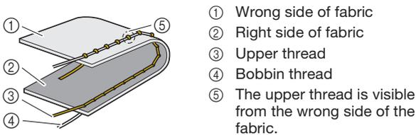
Turn the thread tension dial clockwise to tighten the upper thread tension.
