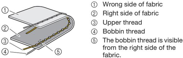
Turn the thread tension dial counterclockwise to loosen the upper thread tension.
