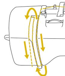
**9** Make sure that the thread is passed into the thread take-up lever as shown below.
