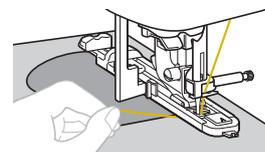
**7 After sewing is finished, raise the presser foot lever, remove the fabric, and then cut the threads.**
