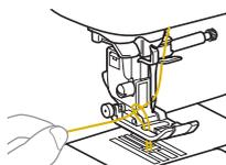
**7** Pull up the bobbin thread, pass it under the presser foot and pull it about 10 cm (4 inches) toward the back of the machine, making it even with the upper thread.
