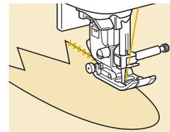
When sewing around corners, stop the machine with the needle in the fabric just outside of the appliqué, raise the presser foot lever, and then turn the fabric as needed to change the sewing direction.
