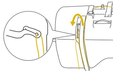
**10** Slide the thread behind the needle bar thread guide.
