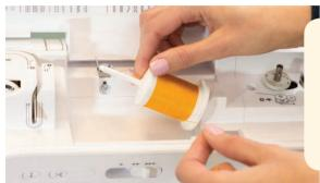
• Place thread on spool pin with thread coming from underneath. Slide on spool cap tightly against thread. Follow the numbered thread path shown on the machine.
