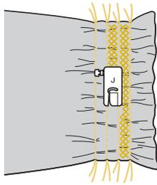
7 Pull out the threads for the straight stitches.
