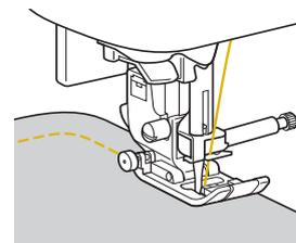
When sewing along a curve while using a zigzag stitch, select a shorter stitch length in order to obtain a finer stitch.
