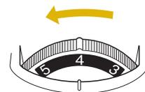
Pushing the thread tension dial toward the right makes the thread tension tighter.
