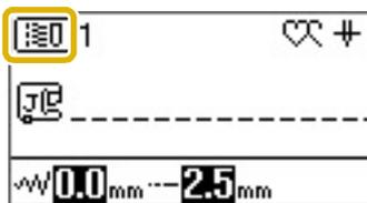
2 Enter the number of the desired stitch using numeric keys.
