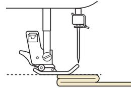
→ After the seam is sewn, the presser foot will return to its original angle.
