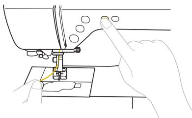
→ The bobbin thread is looped around the upper thread and can be pulled up.
