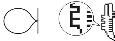
If the pattern appears as shown below, the stitching is misaligned in the vertical direction.
