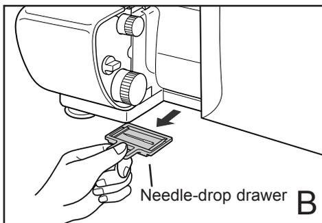
1. Raise the needle to the highest position by turning the handwheel toward you.
