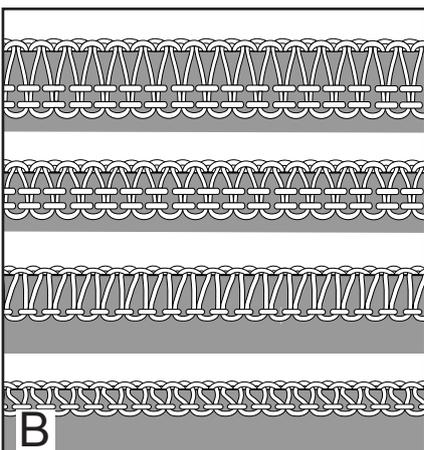
The stitch width is variable by the placement of Right and Left needles and the stitch width dial positions. (Fig. B)
