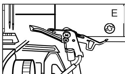
Either needle thread may be engaged for 2-thread overlock sewing.
