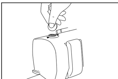
The presser foot pressure has been preset at the factory and rarely needs adjustment. You may find it necessary, however, to decrease the pressure for thick fabrics or increase pressure for thin fabrics to feed more smoothly under the foot. Use a coin to turn the screw on top of the machine.
