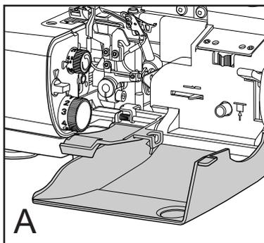
The lower fixed blade is made of a special long-lasting steel and does not require frequent replacement. If necessary, contact your nearest Baby Lock retailer for replacement of this blade.
