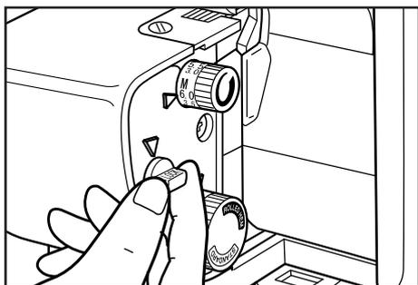
When no trimming is desired, as when stitching on a fold, flip the cutting blade lock switch clockwise to the LOCK position. The cutting blade no longer moves up and down, but remains in its lowered position. To re-engage the cutting blade, turn the cutting blade lock switch half of a turn counter-clockwise. The blade will start moving automatically when you start sewing.
