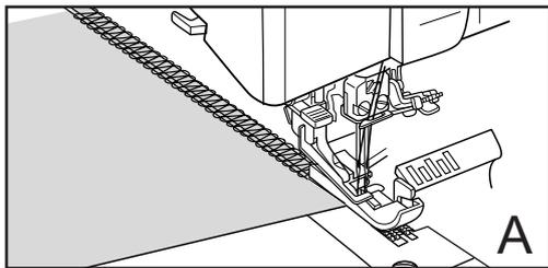
1. Stitch along one edge until you reach the corner. Take one stitch off the edge of the fabric. (fig. A) (As you approach the edge, you may want to stop and manually turn the handwheel towards you.)
