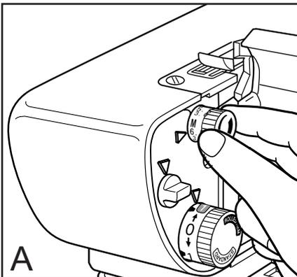
The stitch width adjusting dial is located above the stitch length dial. (fig. A) The stitch width dial displays two sets of numbers, indicating two width ranges. The larger size numbers on the dial, 5.5 through 7.5mm, denote the stitch width when the left needle is in use. The smaller size numbers, 3.0 through 5.0mm, apply when the right needle is in use. The "M" setting (3.5) is for the rolled edge.
