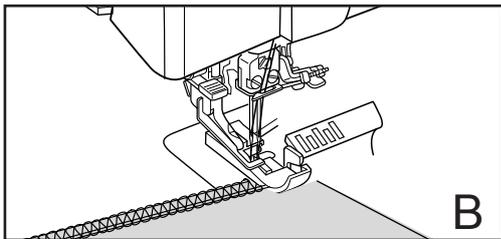
**Note:** A loose thread loop at the corner is caused by too much slack in the needle thread when clearing the stitch fingers. Try again, turning corners takes a little practice!
