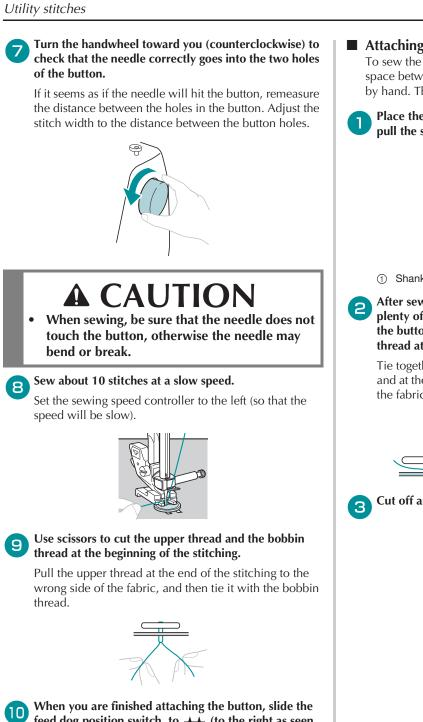
feed dog position switch, to 👬 (to the right as seen from the rear of the machine) and turn the handwheel to raise the feed dogs.
