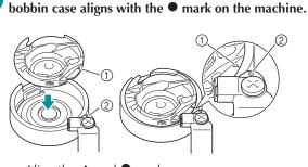
Insert the bobbin case so that the **A** mark on the
