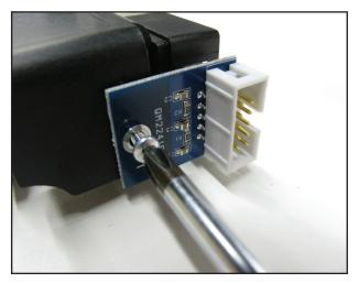
3. Gently pull the circuit board outward toward the front of the quilting machine (the same direction the screw came out).
