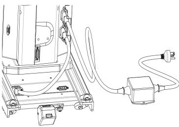
6. The black cables attached to the Pro-Stitcher carriage should be routed up between the rear handles and the quilting machine, toward the right-hand side of the machine (looking at the machine from the back). Attach the cable clips (*see Parts List, item J*) and route the cable accordingly. Plug the other end of the power cord into the back of the quilting machine.
