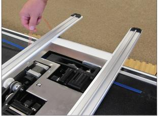
3. Use the carriage as a guide and align the blue Flexirack with the white gear along the length of the table (see arrow at right), removing the pink protective layer and pressing downward on the blue Flexirack while moving down the entire length of the table.
