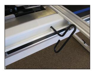
9. With the power cable unplugged and the motors in the engaged position (use the manual engagement/disengagement tool if necessary), ensure that as the quilting machine is moved in both the X and the Y directions, the corresponding gears are rotating as well.
