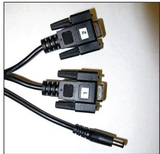
Insert the barrel connector into the center jack located on the bottom edge of the black box that is mounted to the back of the computer bracket. Attach the two 9-pin serial cables to the appropriate ports on the back of the same box, making sure cable connectors are plugged into their corresponding ports on the black box.
