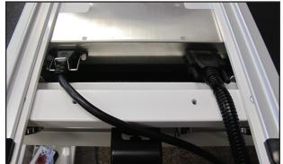
4. Connect one end of the two-foot power cord (*see Parts List, item I-2*) to the carriage power inlet and the other end into the quilting machine's P-pod lower power outlet.
