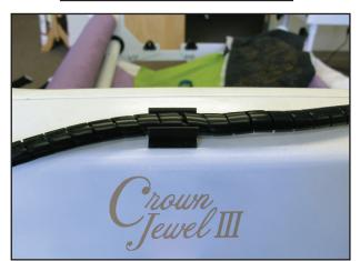
7. The small black cable with the black 3-connector clip should be routed underneath the P-Pod and snapped into the quilting machine's Y-encoder.
