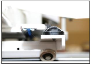
IMPORTANT: If necessary, use the manual engagement/disengagement tool to move the gears so they engage. Insert the end of the tool into the hole at the front of the Pro-Stitcher Carriage.
