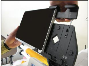
With the computer installed in the bracket, connect the USB short cable (see Parts List, item M) between the USB port, on the top-left side of the computer (position A) and the black box on the back of the bracket (position E).
