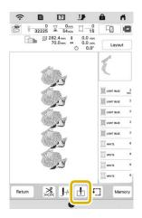
Press to set the starting point to the center top of the pattern.
