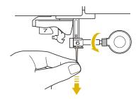
With the flat side of the needle facing the back, insert the new needle all the way to the top of the needle stopper (viewing window) in the needle clamp. Use the disc-shaped screwdriver to securely tighten the needle clamp screw.
