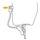
Use the included disc-shaped screwdriver to loosen the screw for the embroidery foot, and then remove the embroidery foot "W+" with LED pointer.
