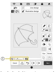
\* After the loaded image is converted to stitching, it appears as a background in the pattern drawing screen. Use gauge ① to adjust the transparency of the background. Each press of 【 lightens the background, making the line pattern darker. Each press of 】 darkens the background, making the line pattern lighter.
