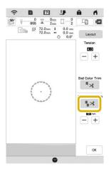
→ The key will display as \[ \frac{1}{2} \simes \]. The machine will not trim the thread before moving to the next stitching.
