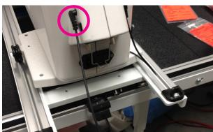
4. Plug the small end of the Pro-Stitcher carriage communication cable (see Parts List, item M) into the top right connector, labeled Pro-Stitcher, on the machine back connection panel.
