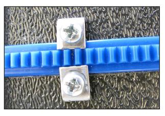
NOTE: As an alternative, use one clamp at each end. Slide the lip of the clamp over the last gear of the blue Flexirack, drill a pilot hole, and screw in place.
