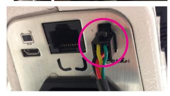
5. Plug the large end of the Pro-Stitcher carriage communication cable (see Parts List, item M) into the back of the carriage (right side as seen from back of machine). Tighten the black screws using a flat-head screwdriver.
