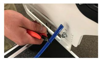
6. At both ends of the blue Flexirack, use two of the small metal clamps (see Parts List, item C) to hold the ends firmly in place. The clamps have a hole through the center and a lip on one end. The lip should be on the side opposite the blue Flexirack. Place the clamps where they will be attached and drill pilot holes using the 3/32-inch drill bit and then use a Phillips screwdriver to fasten the clamps on both sides of the Flexirack to the table.
