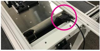
6. Plug the 12' power cord (see Parts List, item I) and into the back of the Pro-Stitcher carriage. Secure the power cord into the Pro-Stitcher carriage by pressing the wire cord-retainer onto the cord.
