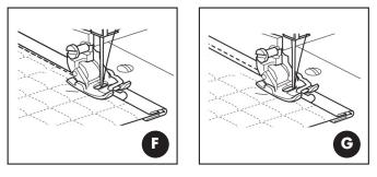
Position the front side of the fabric up, and then sew with the presser foot guide aligned with the edges of the fabric and binding tape.
