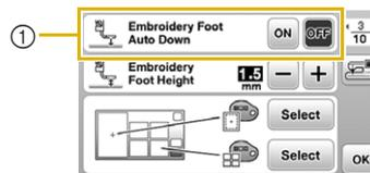
① When set to [ON], pressing the “Start/Stop” button when the presser foot is raised automatically lowers the presser foot before starting embroidering.
