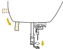
**13** Cut the thread with the thread cutter on the left side of the machine.
