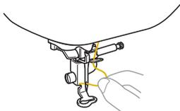
**11** Pull the end of the thread, which has been passed through the needle bar thread guide, to the left, then pass the thread through the notch of the threader thread guide, and then firmly pull the thread from the front and insert it into the slit of the threader thread guide disk marked "7" all the way.
