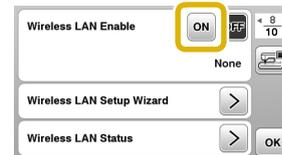
→ The machine prepares for wireless connection.
