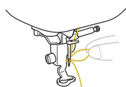
**16** Raise the presser foot lever, pass the end of the thread through and under the presser foot, and then pull out about 10 cm (approx. 4 inches) of thread toward the rear of the machine.
