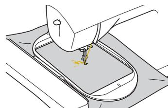
7 Remove the thread for the first color from the machine.
