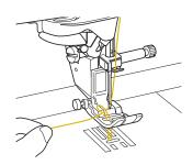
Pull up the bobbin thread, pass it under the presser foot and pull it about 10 cm (approx. 3-4 inches) toward the back of the machine, making it even with the upper thread.
