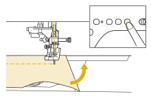
The pivot setting is useful when changing the sewing direction. When the machine is stopped at the corner of the fabric, the machine stops with the needle in the fabric and the presser foot is automatically raised so the fabric can easily be rotated ("Pivoting" on page 82).
