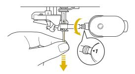
With the flat side of the needle facing the back, insert the new needle all the way to the top of the needle stopper (viewing window) in the needle clamp. Use a screwdriver to securely tighten the needle clamp screw.
