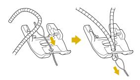
Attach the couching sole for digital dual feed foot shown below to the compact digital dual feed foot.
