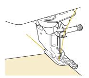
Rotate the handwheel toward you (counterclockwise). Check that the needle does not touch the presser foot.
