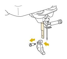
Set the adapter on the presser foot bar, aligning the flat side of the adapter opening with the flat side of the presser foot bar. Align the screw holes in the adapter and presser foot bar, and then securely tighten the screw with the screwdriver.
