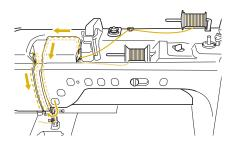
Continue threading; however, do not pass the thread in the needle bar thread guide "6" on the needle bar. Thread the needle on the right side manually.
