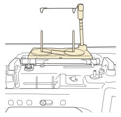
Place the spool of thread on the spool pin so that the thread feeds off the spool clockwise. Firmly insert the spool cap onto the spool pin.
