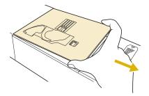
6 Insert the tabs on the straight stitch needle plate into the notches in the machine.
