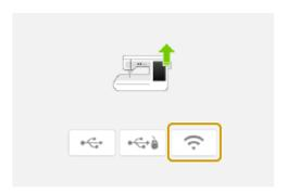
Be sure to NOT turn off your machine while the machine is saving the update software to itself. If the machine's power is turned off while saving the update software, it may result in damage to the machine.
