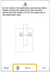
In order to cleanly connect the patterns, make sure that the distance between the embroidery positioning stickers (distance between the centers of the large circles) is the same before and after rehooping the fabric. If the distance is not the same, the fabric may not be taut. At this time, do not correct the distance by moving a sticker.
