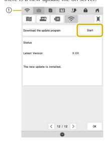
(1) When the wireless LAN key appears as , touching start causes the machine to check if there is a new update file. If there is a new file, downloading begins.
