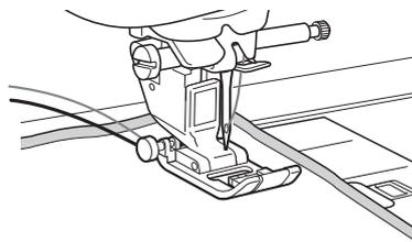
**14** While gently holding threads at the rear of the machine, turn the handwheel to feed the needle into the fabric or punched hole again, and then lower the presser foot lever.
