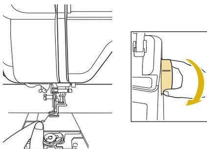
**16** Gently pull the upper thread to bring the bobbin thread up through the needle plate.
