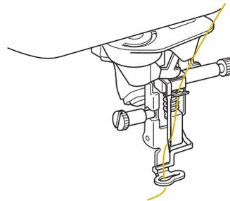
**2** Lower the presser foot, then press the “Start/Stop” button to start embroidering. After 5-6 stitches, press the “Start/Stop” button again to stop the machine.
