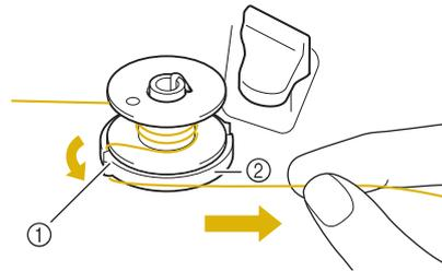
① Guide slit (with built-in cutter)
