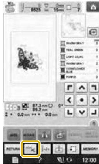
2 Press to turn off the automatic thread cutting function.
