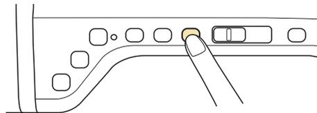
→ The upper thread shutter opens so the machine can be threaded.
