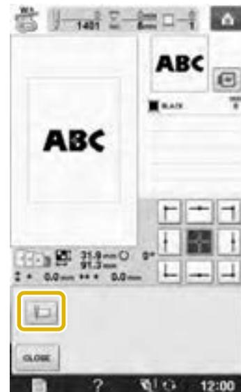
→ The needle is positioned in the lower-left corner of the pattern. The embroidery frame moves so that the needle is positioned correctly.
