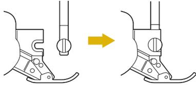
**3** Hold the dual feed foot in place with your right hand, then using the included screwdriver securely tighten the large screw.
