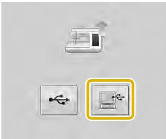
**3** Plug the USB cable connector into the corresponding USB ports for the computer and for the machine.
