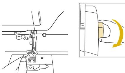
**15** Gently pull the upper thread to bring the bobbin thread up through the needle plate.
