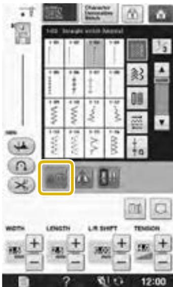
→ The key appears as
