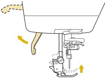
\* If the presser foot is not raised, the sewing machine cannot be threaded correctly.
