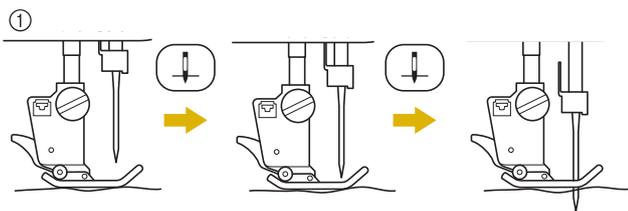
\* When the needle is nearly lowered by pressing the “Needle Position” button, the feed dogs are lowered. At this time, the fabric can be shifted to finely adjust the needle drop position.
