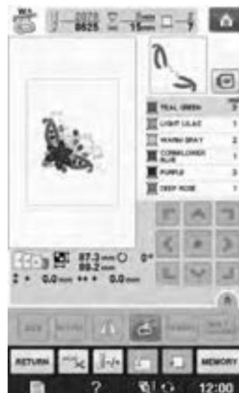
→ When the last color is sewn, “Finished sewing” will appear on the display. Press
