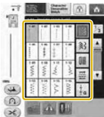
→ The symbol of the correct presser foot will be displayed in the upper left corner of the LCD screen.
