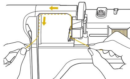
**8** Guide the thread down, up, then down through the groove, as shown in the illustration.
