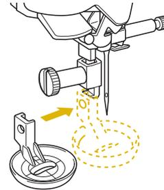
5 Tighten the screw with the included screwdriver.
