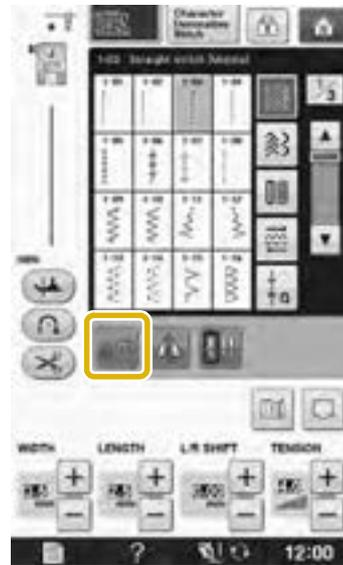
→ The key appears as
