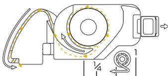
**5** While lightly holding down bobbin with your right hand as shown, guide the thread through the slit (①) and (②).
