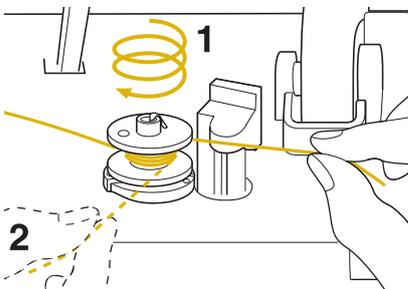
**8** Pass the end of the thread through the guide slit in the bobbin winder seat, and pull the thread to the right to cut the thread with the cutter.
